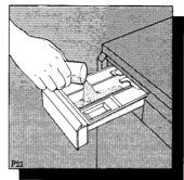
Following the table (page 16), measure the required quantity of washing powder and pour into the compartment f U, the main wash compartment.
